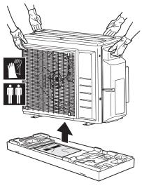
2 Remove the accessories at the bottom of the package.
