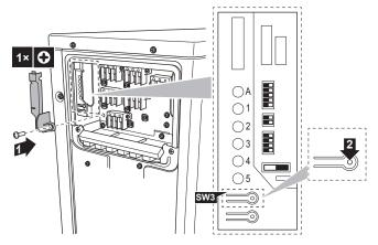
2 Press the wiring error check switch (SW3) on the outdoor unit service PCB.
